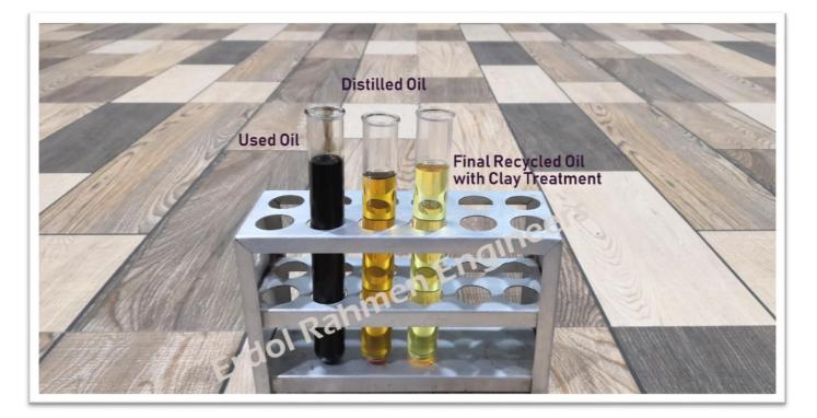
Used Oil > Distilled Oil > Recycled Base Oil (With Clay Treatment method)
