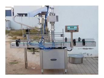
This automatic inline capper is a high speed capper applicable for round, rectangular and most irregular bottles. Machine has a noiseless cap elevator to unscramble and feed caps for capping system. Unique design of machine requires no changeover parts and no tools when changing caps size. Customization available to meet specific requirement by customers.
