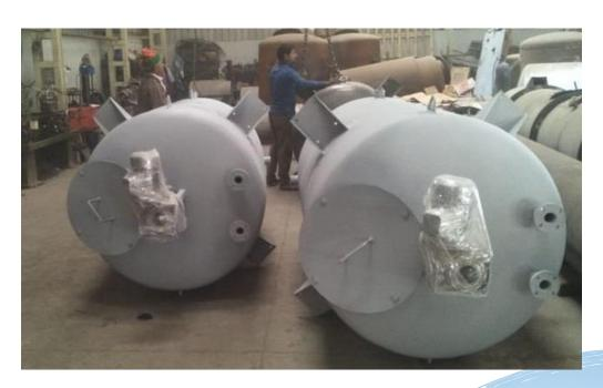
Lubricant blender is used for mixing additives with base oil to formulate Lube oil, thus it can be called main equipment of plant. It has automation for feeding raw materials by load cell & HMI-PLC, mixing and heating arrangements.
