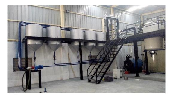
**ERE manufactures Additive storage tanks equipped with:**
