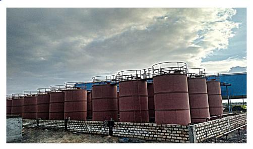
For storing various base oils like - SN 150, SN 500 from mineral base or synthetic base, base oil storage tanks are needed. Size of these storage tank varies depending upon availability of base oil, available area, available initial investment, available working capital etc. ERE manufactures storage tank up to 50000 Liters (13200 US gallons) capacity with Mild Steel or Stainless Steel.
