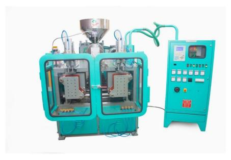
Automatic blow molding machines are needed for making Lube oil bottles, these machine comes with various mechanical customizations according to requirement of production speed. For lube oil industry, 2 machines are recommended - first machine for making Lube oil bottles up to 1 Liter - second machine for making Lube oil bottles up to 5 Liter.
